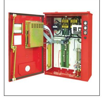
**Description** – Firetrol® combined automatic and manual Mark II based diesel engine fire pump controllers are intended for starting and monitoring fire pump diesel engines. They are available for use with 12 or 24 volt negative ground systems using lead acid or Nickel-Cadmium batteries. The controller monitors, displays and records fire pump system information.
